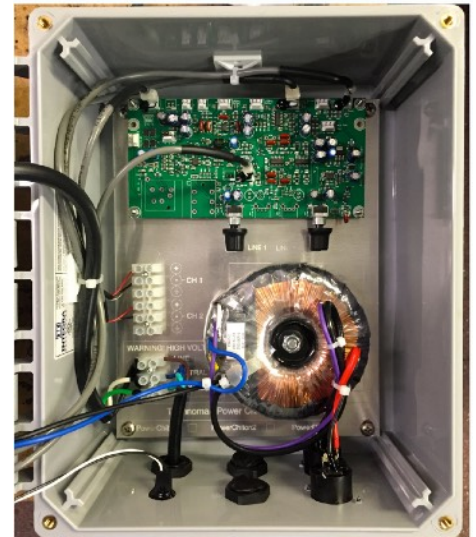
Interior photo of PowerChiton with optional 70V output transformer
